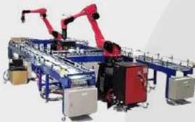
CONVEYOR BELT + ROBOTIC ARM INTEGRATION
